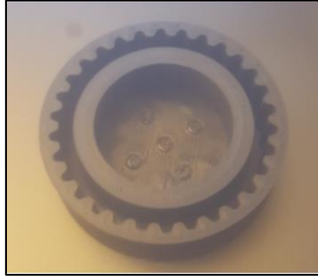
Figure 6.14: Direct Drive Interface for Motor 1
