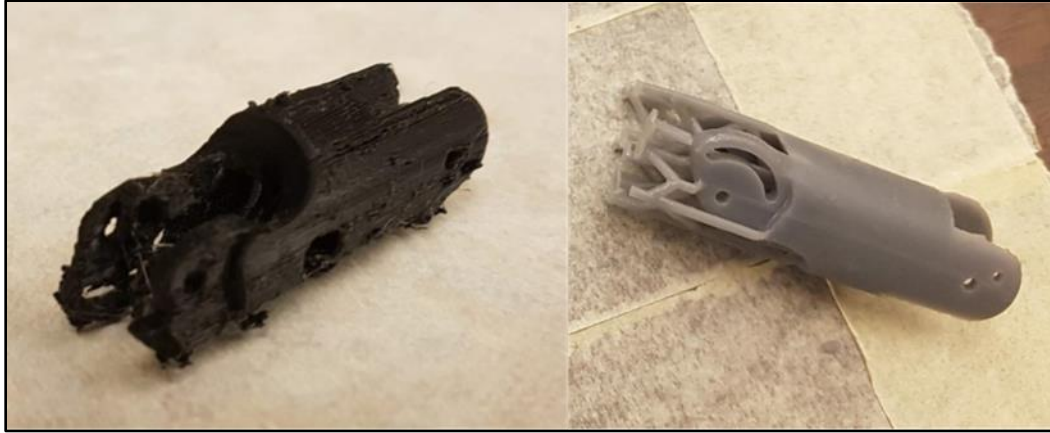
Figure 6.9: Finger Construction Comparison between PETG (Left, Black Color) versus SLA Resin (Right, Grey Color)
