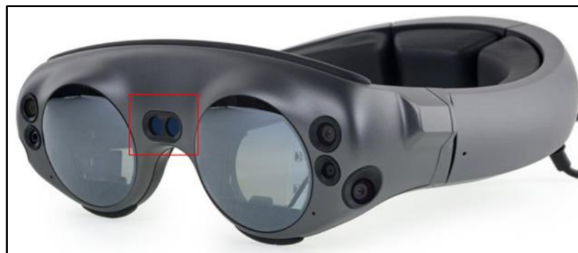
Figure 6.5: IR Projector Location Note: BY-NC-SA-3.0 by Copyright Owner.
