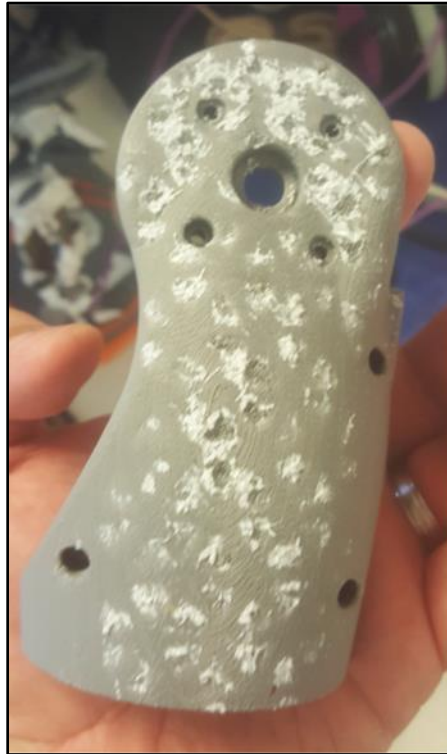
Figure 6.10: ABS Housing with Support Structures from 3D printing Still Fused to the Housing
